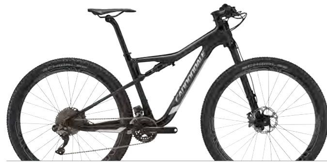
SCALPEL-SI BLACK INC. FRAME New Scalpel-Si, 100mm, BallisTec Hi-MOD Carbon, Ai offset SUSPENSION F/R Lefty 2.0 Carbon XLR / RockShox Monarch XX, 100mm, Full Sprint RD/SHIFT/CRANK Shimano XTR Di2 / HollowGram SiSL2, Praxis rings, 26/36 Ai BRAKES Shimano XTR Race WHEELSET ENVE Carbon M50 w/ Lefty 60 and Chris King hubs, Ai (27.5" Sm, 29" M-XL) COOL BITS ENVE Carbon bar and post / Tubeless Kit COLOR Jet Black w/ Chrome and Cashmere - Satin / Gloss (BLE)
