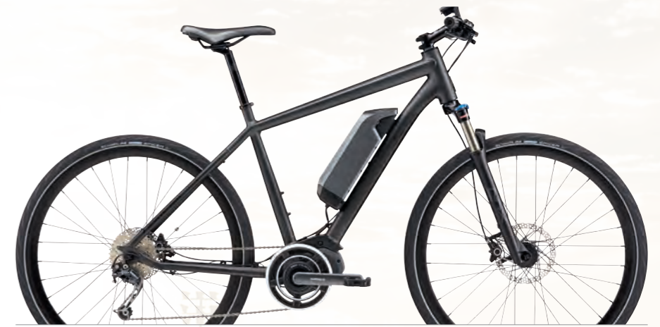
KINNETO FRAME Kinneto Men, SmartForm C3 Alloy FORK SR Suntour NRX-DS, 75mm, lockout DRIVE UNIT / BATTERY Shimano Steps E6000 250W / 418Wh battery GROUP Shimano Deore 9-speed BRAKES Shimano M365 hydro disc COOL BITS Schwalbe Spicer, 700x40c, puncture protect tires with reflective sidewall / Cannondale Fitness Pedals COLOR Matte Nearly Black w/ Jet Black - (GRY)
