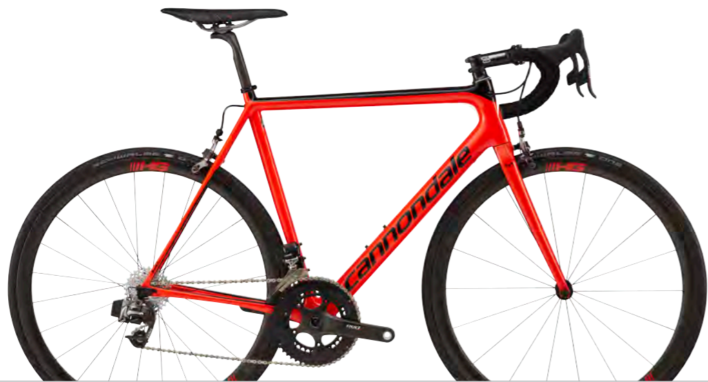
SUPERSIX EVO HI-MOD RED ETAP FRAMESET SuperSix EVO, BallisTec HI-MOD Carbon GROUP SRAM Red eTap CRANKSET SRAM Red, BB30a 52/36 WHEELSET Cannondale HollowGram Carbon Clincher COCKPIT Cannondale Escape Hanger Carbon Bar / C1 Ultralight Stem / SAVE Seatpost with Fi'zi:k Arione R3 Saddle COLORS Acid Red w/ Jet Black - Gloss (ARD)
