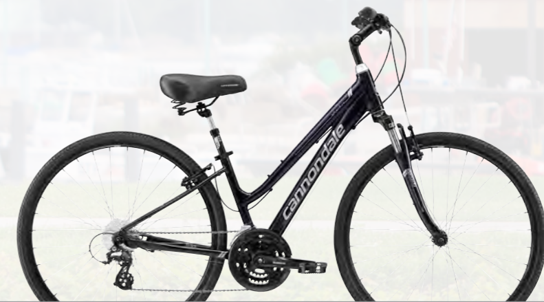
ADVENTURE WOMEN'S 2 FRAME Adventure Women's, Step-Thru, SmartForm C3 Alloy FORK SR Suntour SF-15, 50mm RD/SHIFT/CRANK Shimano Altus/Tourney/Revo Twist BRAKES Cannondale V-Brake w/modulator COOL BITS RST Suspension seatpost, Cannondale Ultra Comfort saddle COLOR Midnight Blue w/ Fine Silver and Powder Blue - Gloss (MDN)
