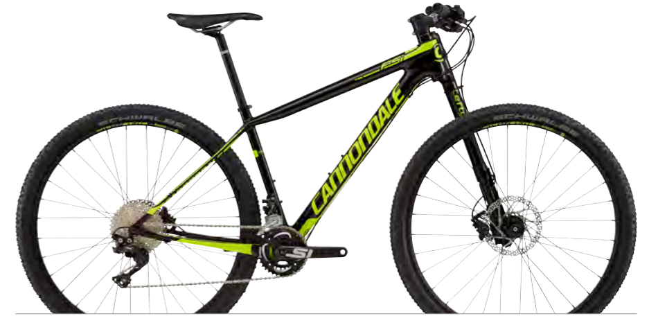
F-Si CARBON 4 FRAME F-Si, BallisTec Carbon, Ai Offset FORK Lefty 2.0 PBR, 100mm RD/SHIFT/CRANK Shimano XT-SLX / Cannondale Si, 26/36 rings, Ai (27.5" Sm, 29" M-XL) BRAKES Shimano Deore hydro disc WHEELSET WTB STP i19, tubeless ready COOL BITS Cannondale C3 Cockpit / Prolog K3 saddle COLORS Jet Black w/ Neon Spring - Gloss (BLK)
