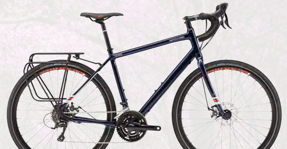
TOURING 2 FRAMESET Touring, SmartForm C2 Alloy GROUP Shimano Sora / Promax Render R disc CRANKSET Shimano Sora, BSA, 50/39/30 WHEELSET DC3.0 Disc / Cannondale C3 hubs COCKPIT Cannondale C3 Touring Bar, C3 Stem/Seatpost with WTB Silverado Comp saddle COLOR Midnight Blue w/ Acid Red and Matte Reflective Silver - Gloss (MDN)
