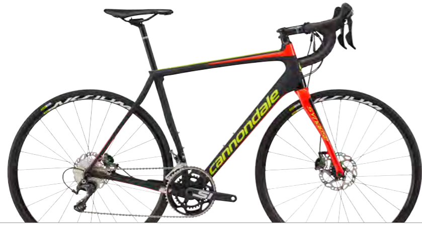
SYNAPSE CARBON DISC ULTEGRA FRAMESET Synapse Disc, BallisTec Carbon GROUP Shimano Ultegra / R685 Disc CRANKSET Cannondale Si w/ FSA rings, 50/34 WHEELSET Mavic Aksium Disc WTS COCKPIT Cannondale C2 Compact Bar/Stem, C3 Seatpost, Selle Royal S1 saddle COLOR Jet Black w/ Volt and Acid Red - Matte/Gloss (VLT)
