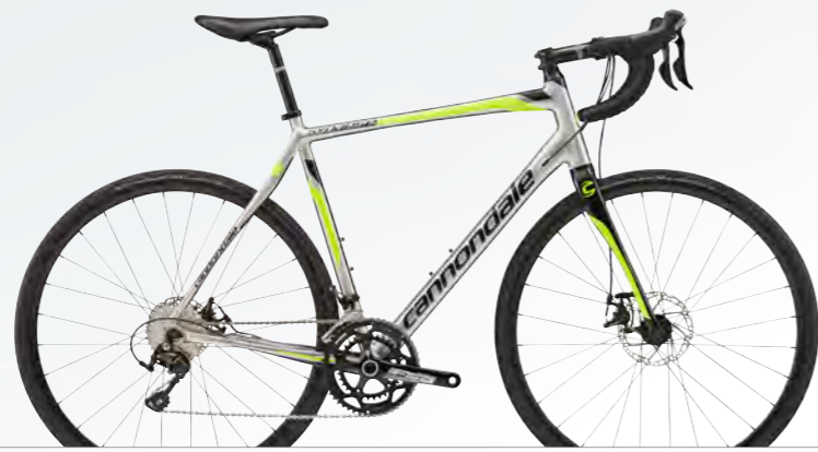
SYNAPSE DISC 105 FRAMESET Synapse Disc, SmartForm C2 Alloy / SAVE carbon bladed fork GROUP Shimano 105 / TRP Spyre C Disc CRANKSET FSA Gossamer, BB30, 50/34 WHEELSET RD 2.0 Disc / Formula Disc hubs COCKPIT Cannondale C3 Compact Bar/Stem/Seatpost with Cannondale Stage Ergo saddle COLOR Brushed Aluminum w/ Nearly Black and Volt - Gloss (RAW)
