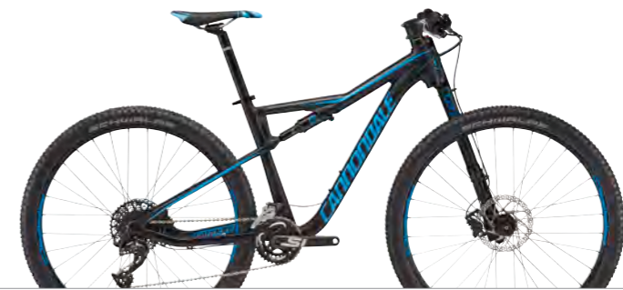
SCALPEL-SI 5 FRAME New Scalpel-Si, 100mm, SmartForm C1 Alloy, Ai offset SUSPENSION F/R Lefty 2.0 XLR / RockShox Monarch RL, 100mm RD/SHIFT/CRANK SRAM GX, S-Series / Cannondale Si, 26/36 rings (Ai) BRAKES Shimano Deore hydro disc WHEELSET Stan's NoTubes ZTR Rapid, Ai (27.5" Sm, 29" M-XL) COOL BITS Cannondale C2 bar / Locking Grips COLOR Matte Jet Black w/ Matte Ultra Blue and Gloss Black (BLK)
