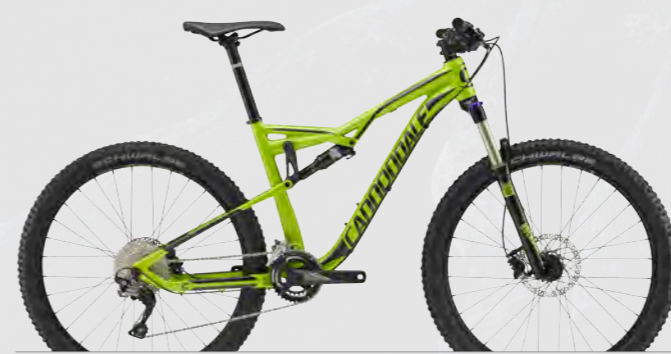
HABIT 5 FRAME Habit, 120mm, SmartForm C1 Alloy SUSPENSION F/R RockShox Recon Gold RL Air / Monarch RT, 120mm RD/SHIFT/CRANK Shimano SLX / FSA Comet MegaExo, 36/26 BRAKES Shimano M447 hydro disc WHEELSET WTB STP i23 - 27.5" COOL BITS Schwalbe Nobby Nic tires, 2.35 F / 2.25 R COLOR Acid Green w/ Anthracite - Gloss (AGR)
