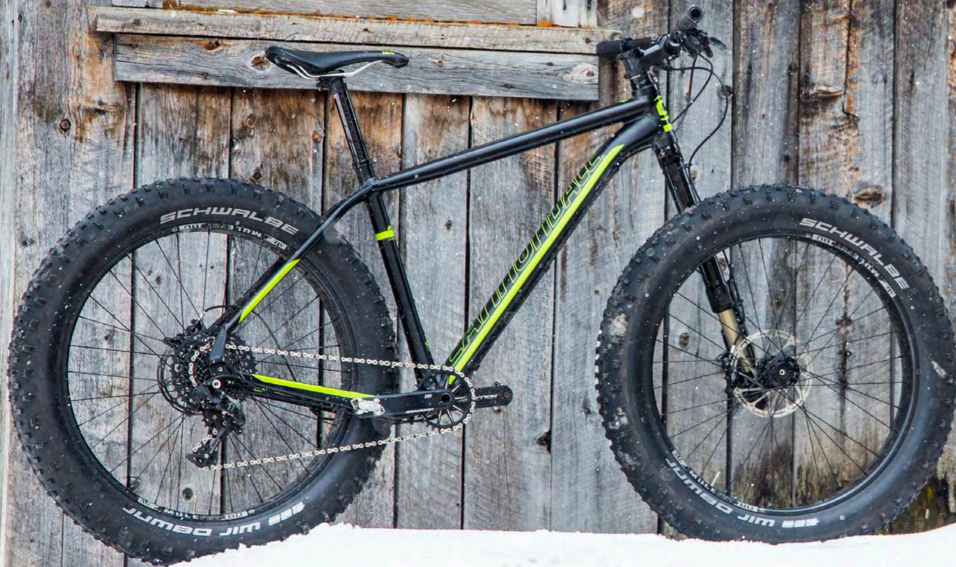
FAT CAAD 2 FRAME Fat CAAD, SmartForm C1 Alloy FORK Cannondale Fatty-Fat Rigid, 55mm offset RD/SHIFT/CRANK SRAM X7-X5 / Cannondale Si, Ai Offset Spider, 34/24 BRAKES SRAM Guide R WHEELSET Sun Ringle Mulefüt 80 SL / Schwalbe Jumbo Jim 26x4.8" COOL BITS Cannondale C3 Cockpit / WTB Silverado Comp saddle COLOR Matte Green Clay w/ Gloss Reflective Silver, Acid Red (GCL)
