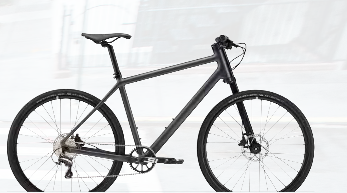
BAD BOY 2 FRAME New Bad Boy OPI, SmartForm C1 Alloy FORK Lefty LightPipe w/ integrated LED light RD/SHIFT/CRANK Shimano Metrea 1x11 / Cannondale Si w/ SpideRing 38t COOL BITS Schwalbe G-One Performance 650x40c tires / Integrated seatpost rear light / Integrated Stem COLOR Nearly Black w/ Charcoal Gray and 3M Reflective - Matte (BBQ)
