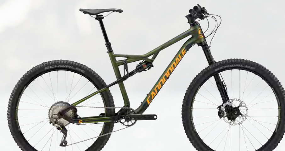
HABIT CARBON 2 FRAME Habit, 120mm, BallisTec Carbon SUSPENSION F/R Lefty 2.0 XLR / RockShox Monarch DebonAir XX, 120mm - Full Sprint RD/SHIFT/CRANK Shimano XTR-XT / HollowGram Si, 30t SpideRing BRAKES Shimano XT WHEELSET Stans Arch Ex MK3 - 27.5" COOL BITS Fox Transfer dropper / Cannondale C1 Carbon bar COLOR Vulcan Green w/ Acid Orange, Jet Black - Matte (VUG)
