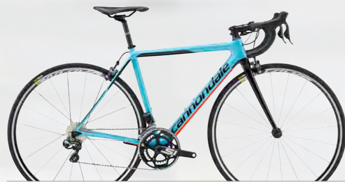
SUPERSIX EVO WOMEN'S ULTEGRA Di2 FRAMESET New SuperSix EVO Women's, BallisTec Carbon GROUP Shimano Ultegra Di2 CRANKSET Cannondale Si w/ FSA rings, 50/34 WHEELSET Mavic Aksium WTS COCKPIT Cannondale C3 Wing Bar/Stem, C2 Carbon seatpost with Selle Royal Seta S1 Women's saddle COLOR Surf Blue w/ Jet Black and Acid Red - Gloss (SRF)
