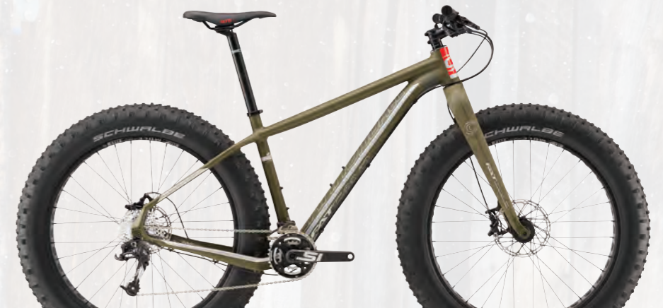
FAT CAAD 2 FRAME Fat CAAD, SmartForm C1 Alloy FORK Cannondale Fatty-Fat Rigid, 55mm offset RD/SHIFT/CRANK SRAM X7-X5 / Cannondale Si, Ai Offset Spider, 34/24 BRAKES SRAM Guide R WHEELSET Sun Ringle Mulefüt 80 SL / Schwalbe Jumbo Jim 26x4.8" COOL BITS Cannondale C3 Cockpit / WTB Silverado Comp saddle COLOR Matte Green Clay w/ Gloss Reflective Silver, Acid Red (GCL)
