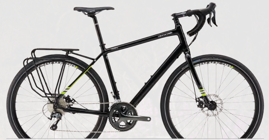
TOURING 1 FRAMESET Touring, SmartForm C2 Alloy GROUP Shimano Tiagra / SRAM BB7 cable disc CRANKSET Shimano Tiagra, BSA, 50/34 WHEELSET DC3.0 Disc / Cannondale C3 hubs COCKPIT Cannondale C3 Touring Bar, C3 Stem/Seatpost with WTB Silverado Comp saddle COLOR Jet Black w/ Berserker Green and Magnesium White - Gloss (BLK)
