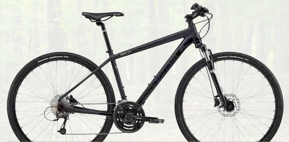
QUICK CX 3 FRAME New Quick CX, SmartForm C2 Alloy FORK SR Suntour NCX, tapered, lockout, 50mm RD/SHIFT/CRANK Shimano Deore-Alivio / Acera, 48/36/26 WHEELS/TIRES Maddux DC 4.0 / Panaracer Comet Hardpack, 700x38c COLOR Midnight Blue w/ Gloss Jet Black and Neon Spring Gloss / Matte (MDN)
