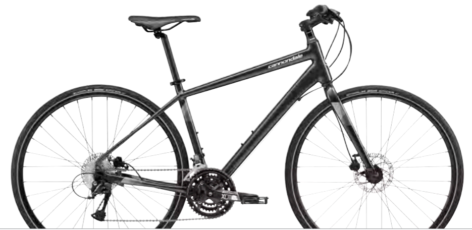
QUICK 5 DISC FRAME New Quick Disc, SmartForm C3 Alloy, SAVE FORK New Quick Disc, SmartForm C3 Alloy, 1-1/8" steerer RD/SHIFT/CRANK Shimano Acera - Altus / Suntour XCM, 48/36/26 WHEELS/TIRES Cannondale C4 / Schwalbe Spicer w/Puncture Protection and Reflective, 700x35c COLOR Nearly Black w/ Magnesium White, Fine Silver, Reflective Detail - Gloss (NBL)
