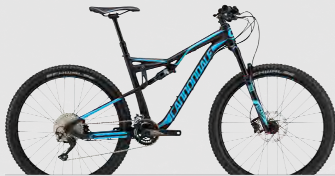
HABIT 4 FRAME Habit, 120mm, SmartForm C1 Alloy SUSPENSION F/R RockShox Revelation RL / Monarch RT, 120mm RD/SHIFT/CRANK Shimano SLX / FSA Comet MegaExo, 36/26 BRAKES Shimano Deore hydro disc WHEELSET WTB STP i23 - 27.5" COOL BITS Schwalbe Nobby Nic tires, 2.35 F / 2.25 R, TransX internal dropper post COLOR Jet Black w/ Ultra Blue - Matte (BBQ)
