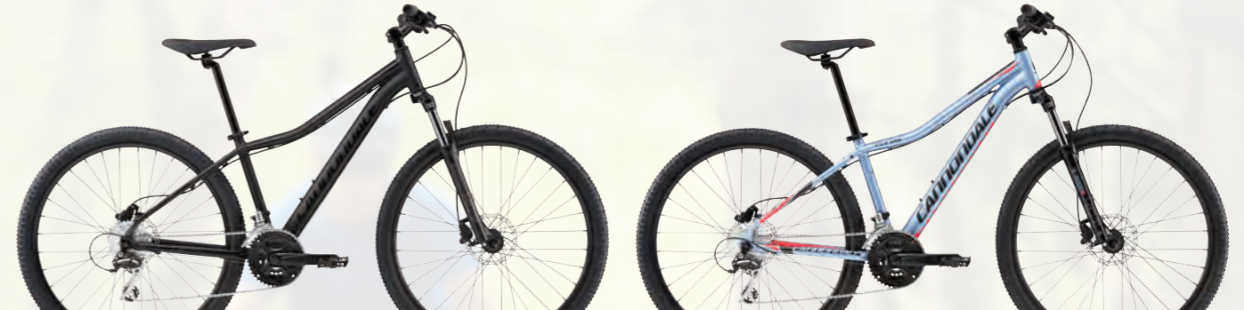
FORAY 2 FRAME Foray, SmartForm C3 Alloy FORK SR Suntour XCT-100, 100mm, coil RD/SHIFT/CRANK Shimano Acera-M310 Rapidfire Plus / Prowheel, 24/34/42 BRAKES Tektro M285 Hydro Disc WHEELSET Alex DC 6.0 - 27.5" COOL BITS Cannondale C-Series cockpit / Stage 2 Women's Saddle COLOR Matte Jet Black w/ Gloss Jet Black - (BBQ) / Powder Blue w/ Nearly Black, Acid Strawberry - Gloss (BLU)
