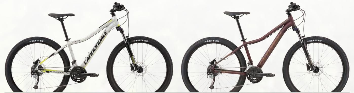
FORAY 1 FRAME Foray, SmartForm C3 Alloy FORK SR Suntour XCM-HLO, 100mm, coil, lockout RD/SHIFT/CRANK Shimano Acera / Shimano M371, 44/32/22 BRAKES Tektro M285 Hydro Disc WHEELSET Alex DC 5.0 - 27.5" COOL BITS Cannondale C-Series cockpit / Stage 2 Women's Saddle COLOR Primer Grey w/ Jet Black, Neon Spring - Gloss (PRM) / Mulberry w/ Dark Gold, Green Clay - Matte (BLO)
