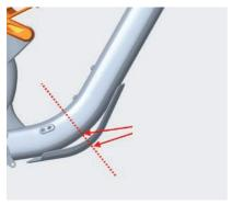
Align center of protector bend with downtube bend. Center on tube.
