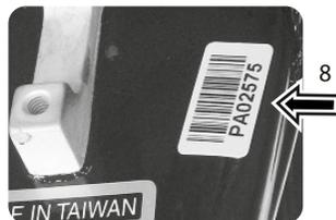
Remove the battery to locate the Bike Serial Number (8).
