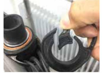
Bend spacer inwards to route cables through first slot, then route cables through the second slot.
