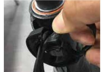
Assemble spacer on steerer tube.
