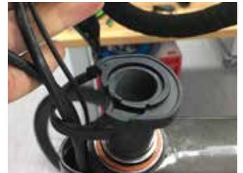
Spacers and stem have interlocking feature to ensure alignment.
