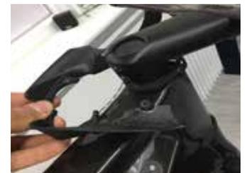
Assemble the stem covers with the M3 bolt (2 Nm)
