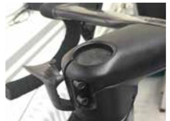
Close right stem cover first, then rotate left stem cover in place and close around the stem body
