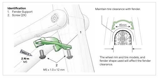
Please Note: (1) Check tire clearance with the tire fully inflated. (2) Mounting a tire with a smaller profile, one smaller than the maximum tire size for the frame, or currently on the wheel may be required to fit a compatible fender. (3) Any fender must be secured by the support and should not be loose. (4) Do not modify any parts or the frame in order to install a fender.
