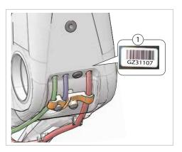
The serial number is located on the bottom bracket. It is a 7-character barcode (1). Use this serial number to register your bike.
