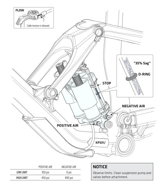
Disconnecting the pump results in very small pressure loss. To determine actual loss for your pump, set pressure, disconnect and reconnect. You can compensate by adding the loss to the table values.
