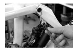
A frame guard should be placed so that the cable does not rub the frame.
