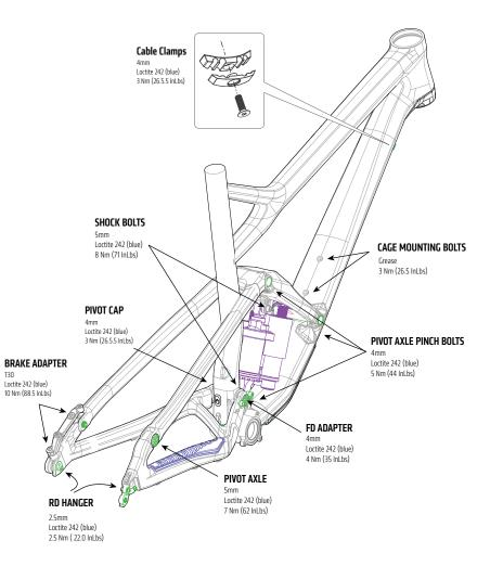
Correct tightening torque for the fasteners (bolts, screws, nuts) on your bicycle is very important to your safety, the durability and performance of your bicycle. We urge you to have your Dealer correctly torque all fasteners using a torque wrench. If you decide to tighten fasteners yourself always use a good torque wrench!
