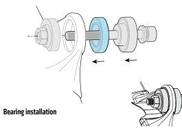
Use **KP169/** tool to install pivot and main shim together. Make sure both are seated against bearing inner race before tightening pinch bolts. Adjust the pivots with the tool so the gap between bearing and link is the same on each side.
