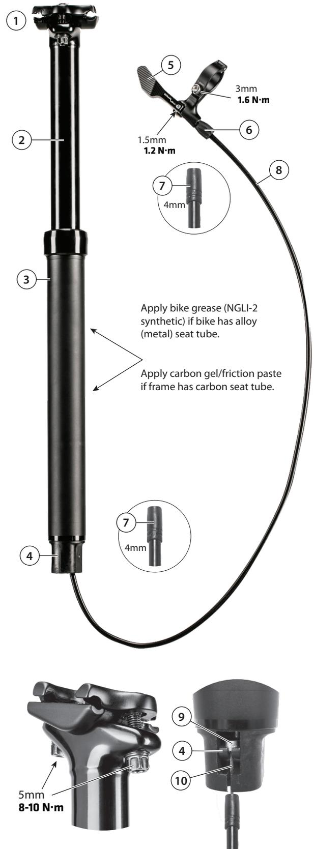
6. Using a thin coating of friction paste for carbon frames and NGLI-2 synthetic assembly grease for metal frames on the outer tube of the post.
