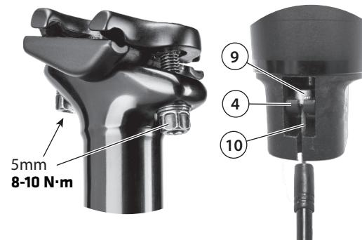
6. Using a thin coating of friction paste for carbon frames and NGI-2 synthetic assembly grease for metal frames on the outer tube of the post.
