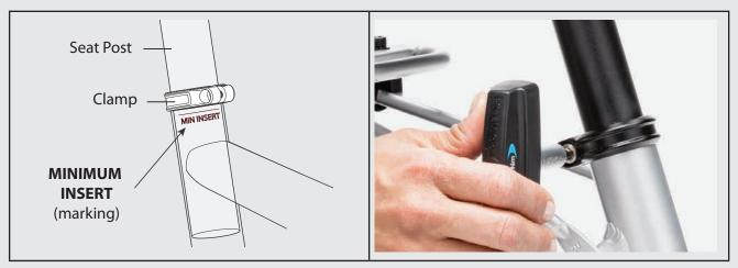
WARNING: All seatposts have a "MINIMUM INSERT" marking. This line must be below the top of the clamp, inside the seat tube and not visible, at all times. Do not ride without adjusting the seatpost height and securely tightening the seatpost clamp bolt or quick-release clamping mechanism. For more information on installation and adjustment of the seatpost, refer to the Owner's Manual.
