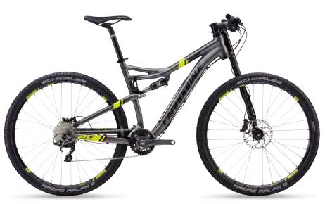
FRAME: Scalpel 29, SmartFormed Alloy SUSPENSION R/F: RockShox Monarch RL (100mm) / Lefty PBR 100 29 (100mm) RD/FD/SHIFT: Shimano SLX/Deore/SLX WHEELSET: Stan's ZTR Rapid 29 BRAKES: Shimano Deore COLOR: Charcoal Grey, w/ Black, Neon Spring - Matte (01)
