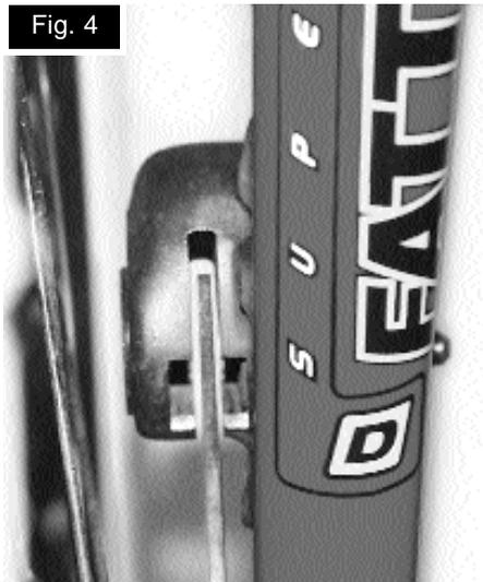
**QBDC/)** PER MONTARE I TUBI DEL FRENO AI FERMA GUAINA DELLA BICI. ASSICURARSI, INOLTRE, CHE I TUBI DEI FRENI NON SIANO TROPPO LUNGI O CHE POSSANO COSTITUIRE UN OSTACOLO PER IL CONDUCENTE. VEDI, PIÙ SOTTO, LA SEZIONE RELATIVA ALL'ACCORCIAMENTO DEI TUBI DEI FRENI.
