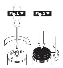
3. While pushing down on the Damping Dial, tighten the 3mm Allen set screw (See Fig. 2.) When properly adjusted, the tuning shaft should stop when the damping dial is turned all the way to the right, providing maximum damping. Note that the Super FT80 and FT70 cartridges do not provide lockout of the suspension.
