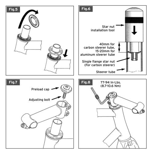
7. Make sure that the top of the steerer tube sits below the top of the stem steerer clamp by 2-3mm. If it is necessary to shorten the steerer tube, mark the steerer tube where it exits the top of the stem. Then use a hack saw and threadless steerer cutting guide to trim the steerer tube 2-3mm below the mark that you made.
