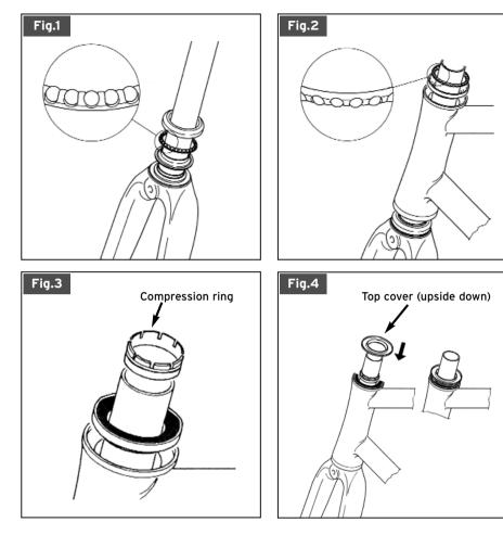
1. Open both bearing cartridges and grease the bearing retainers using a good quality bicycle bearing grease. Reassemble the lower bearing cartridge with the bearing retainer oriented as shown in Fig. 1. Install the lower bearing cartridge on the fork.
