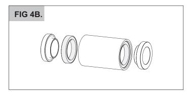
6. Insert the bearing press through the parts as before and press the bearing into the bottom bracket. Remove the tools and press.
