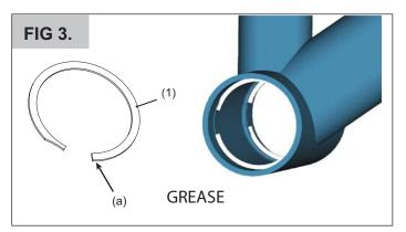
3. Lightly grease the inside of the bottom bracket shell up to
