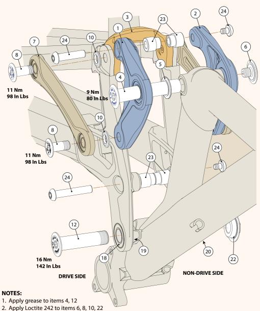
3. Items 10, 19, 20 ridged side (a) face bearing, smooth side (b) face out. 4.Item23,theshockbushings,areavailableonlythroughtherearshockmanufacturer.
