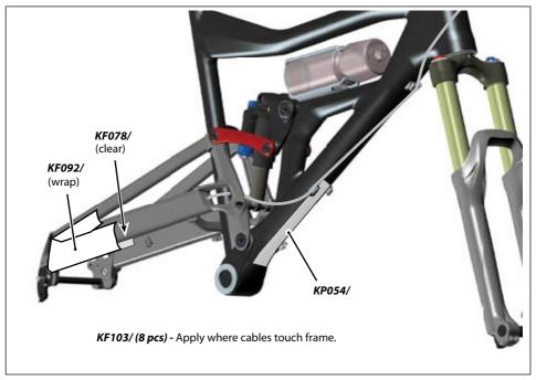
Cable rub can damage your bike frame. Check the line and cable paths over your bike frame after your first few rides. Look for signs of rubbing. Apply guard material on the frame where rubbing is found. When applied correctly, the guards material is good protection for your bike. The illustration above shows typical guard locations on the frame. Replace protection if if it becomes missing or damaged.
