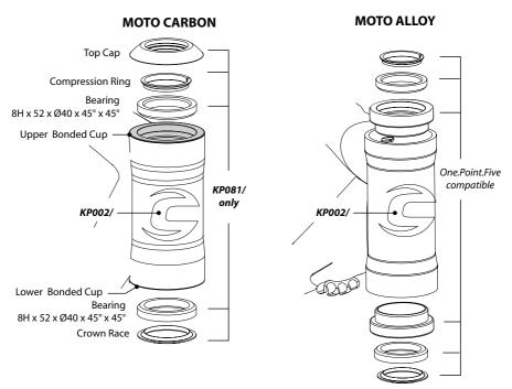
**MOTO CARBON** frames feature permanently bonded headset bearing cups (above left). The cups accept only the Cannondale headset bearing in the kit shown above. The headset kit is compatible with 1.5" steerers.
