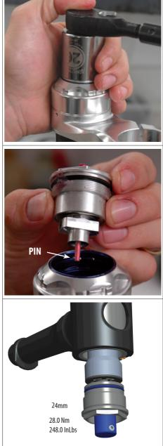
5. Fill the compression valve assembly with the specified fork oil. See **SPECIFICATIONS**.
