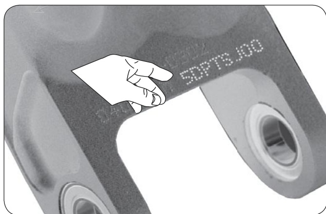
Figure 1 - Code Location (Rear View Of Swingarm Main Pivot)
