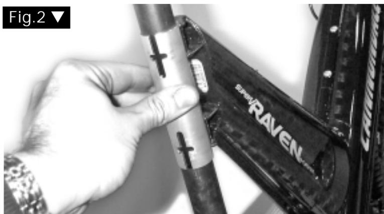
5. With the bolts removed from the two new band clamps, snap the clamps over the sleeve from the back, so that the two tabs on the inside of the band clamps correspond with the widest part of the slots in the back of the sleeve. The clamps have two barrel shaped nuts, one of which is threaded. The threaded side of each clamp should be on the left side of the bike. Pinch in the ends of each band clamp to hold the clamp in place on the back of the seat mast. **See Fig 3.**
