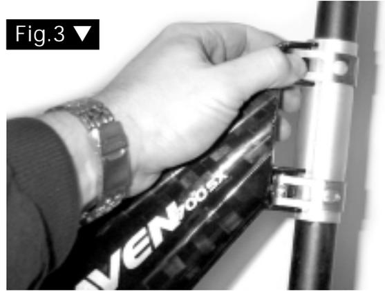
6. Make sure that the seat post extends completely through the aluminum sleeve, but does not interfere with the rear shock or swingarm. If you cannot achieve a tall enough saddle height and still have the seat post extending below the bottom of the sleeve, you must use a longer seat post. **If you cannot achieve a low enough saddle height without having the bottom of the seat post interfere with the rear suspension, you must cut off the bottom of the seat post.**
