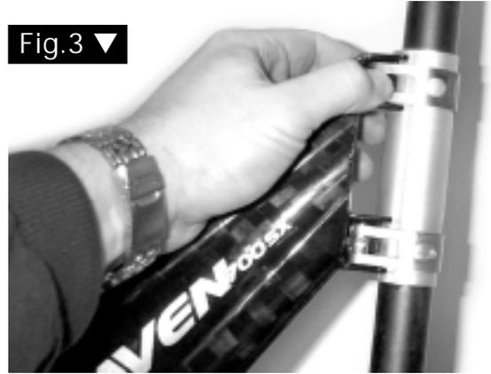
6. Make sure that the seat post extends completely through the aluminum sleeve, but does not interfere with the rear shock or swingarm. If you cannot achieve a tall enough saddle height and still have the seat post extending below the bottom of the sleeve, you must use a longer seat post. **If you cannot achieve a low enough saddle height without having the bottom of the seat post interfere with the rear suspension, you must cut off the bottom of the seat post.**
