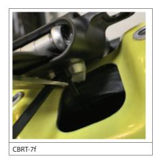
g. The cable sleeve and foam tube should be checked for wear at least once per season. If significant wear is seen, replace the affected components.
