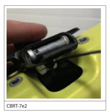
f. Tighten the zip tie, holding the end of the zip tie off to one side of the frame. Tighten the zip tie until it is snug around the cables and hose. Clip the end of the zip tie and proceed the install the tool holder to the frame.
