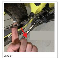
f. Confirm the chain guide does not rub while the rider is pedaling the bike in the largest cassette cog, with the correct sag at the shock (sag at the shock is 10mm).
