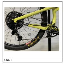
b. Align the chain guide so that it is perpendicular (90 degrees) to the chain.
