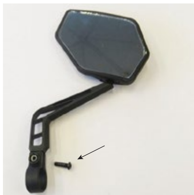
Mounting bracket with M5 × 18mm button head bolt. Torque = 2-2.5 Nm
