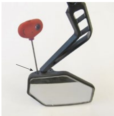
If mirror is loosened after usage you can tighten it again. Maximum torque = 0.8 Nm
