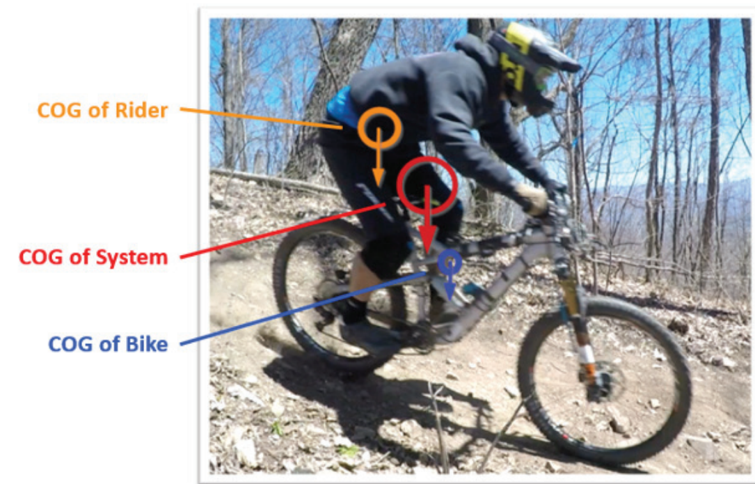
Figure 16 - Test rider on instrumented bicycle with approximate centers of gravity shown.
